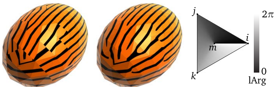
Figure 13. In triangles containing zeros, piecewise linear interpolation ( left ) can be substantially improved ( middle ) by using a closed-form, nonlinear interpolant ( right ).
