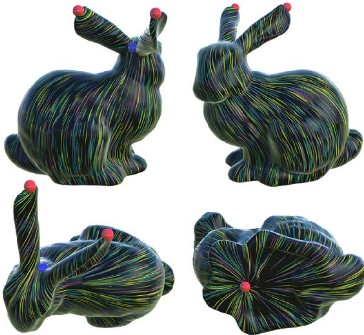
Figure 1. Smoothest unit vector field on the Stanford bunny over all possible configurations of singularities, computed by solving a single eigenvector problem. Red and blue spheres indicate positive and negative singularities, respectively. (471ms, |T| = 28k )
