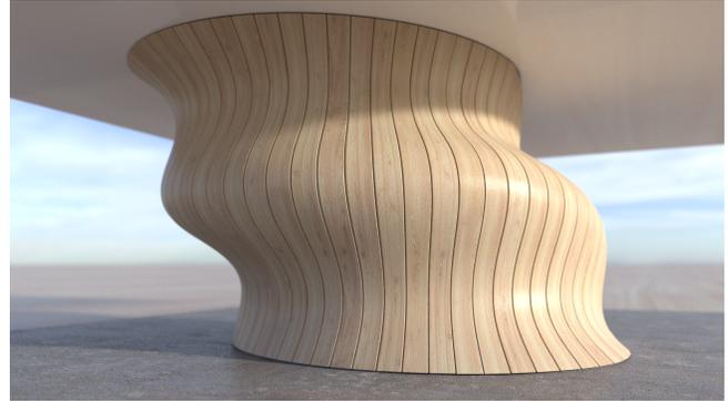
Fig. 2. Rendering of a wooden wall cladding. The underlying surface is isometric to a surface of revolution. It can be realized by attaching a sequence of bent timber strips. All strips develop to the same planar shape.
